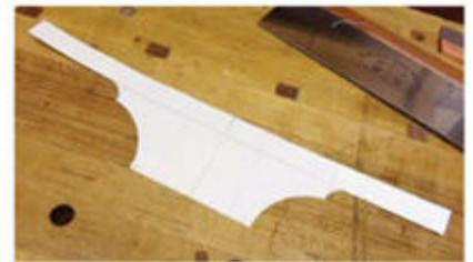
**Shape shifter.** A custom template for your vise jaws allows you to play with a multitude of shapes and configurations. Find one that accommodates all of your saws while leaving mass in the center where it's needed.
