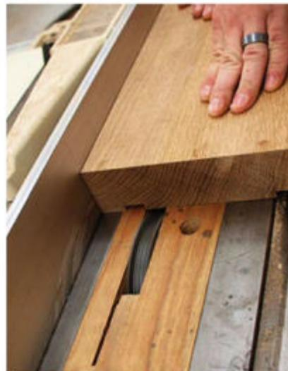
**Quick work.** Hogging out the excess using a stacked dado set is the most efficient stock removal method to create the jaw's recess.
