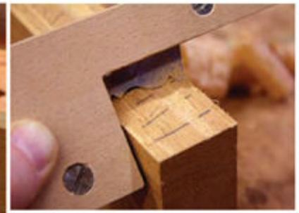
**Fading in.** It's hard to start the profile on the very edge so I just fade it in. As you progress, the pencil marks will be scraped away.
