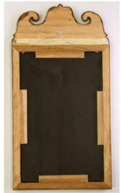
**Blocked in.** Apply a glue block in the rabbet on each of the four sides to hold the glass in place.
