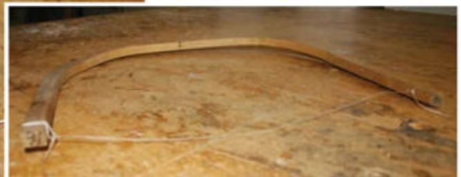
**Delamination & roll up.** A delamination failure (left) – where the part separates along the grain – is common. A roll up failure (above) refers to the piece not remaining flat in the proper plane as it dries. Notice how it lifts off the surface at the top right.
