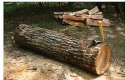
**Split pieces.** Riven logs (in this case, red oak) yield pieces that are split along the grain line, with no runout.
