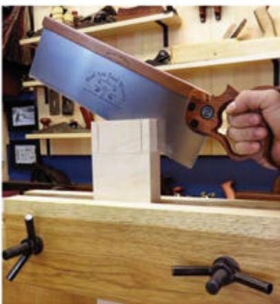
**Moxon moxie.** Using a Moxon-style vise to elevate the work, I cut the tenons by hand. (Use your excess Acme thread to make one of these devices; you won't regret it.)
