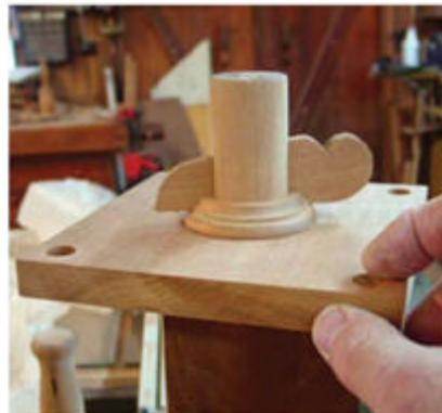
**Fit to turn.** Test-fit the lower plate, washer and key and give it a spin (it should be a tight fit at this point).
