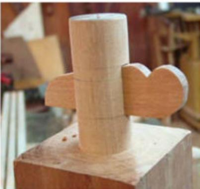
**Key fit.** Plane or sand the sides of the wedge key to not only a nice finish, but to a good, snug fit in the key mortise.
