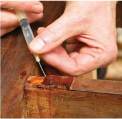
**Crystallize hide glue.** Veneer glued on with animal hide glue is usually easy to crystallize by inserting alcohol under the veneer. I find a syringe to be useful for directing the alcohol.
