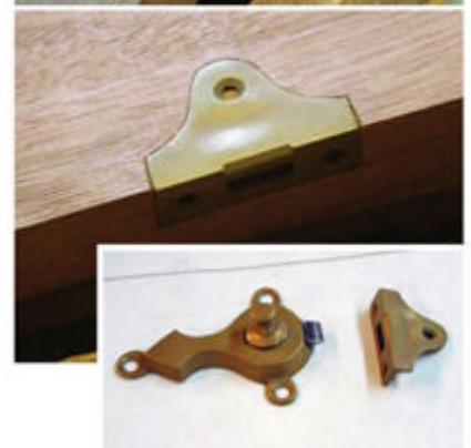
**Latch mortise.** You'll need a latch to keep things in place; the one you choose should have a keeper for the tongue. Mortise that into the top face of the upper plate.
