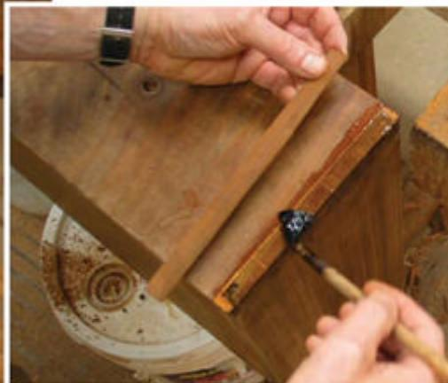
**Veneer patch.** There was nothing to do about the weakness of the bonds to end grain. It's the nature of the way these dovetails were cut. So I trimmed pieces of solid wood with a closely matching grain pattern perfectly straight on one edge with a block plane, then glued them into place, butted tightly against the existing veneer. After the glue dried, I trimmed the excess.
