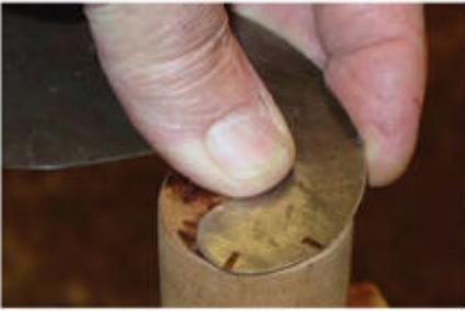
**Arc marks.** A curved scraper can be marked to establish the curve of the spindle. Then use the scraper to scrape a spindle-support trough in a piece of scrap.
