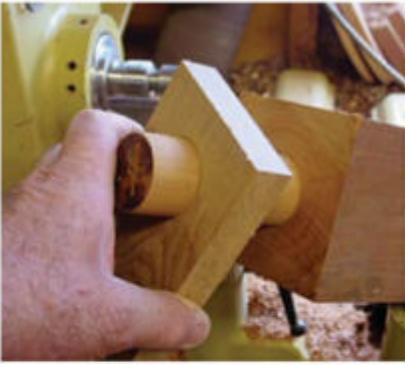
**Strive for perfection.** Use a test block to fit the tenon. It should be just snug enough to spin freely, and be perfectly square to the bottom of the shoulder – check it with an adjustable square.
