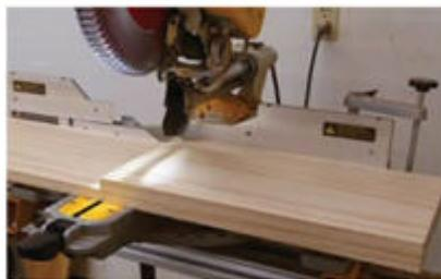
**Matched sets.** Measure, mark, then cut the first shelf and use it to lay out the length of the second shelf. Do the same for the two sides.
