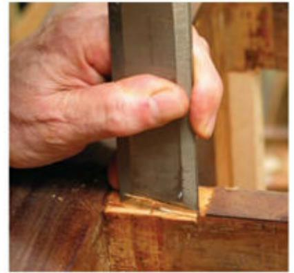
**Build out substrate.** Often the drawers have worn into the front rail of the chest so that the wear has to be built out before the veneer can be replaced. Here, I'm using a chisel to cut a flat surface for the patch to be glued on to.
