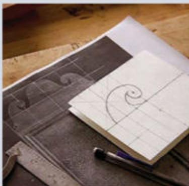
**Box it in.** Start by cutting a piece of posterboard to the exact width and height of the fretwork. Because the design is symmetrical, you can then fold the paper in half lengthwise. You will only be drawing one half of the design. This way, if your cutting is a little off somewhere, everything is still perfectly symmetrical. Don't waste your time drawing this design twice.
