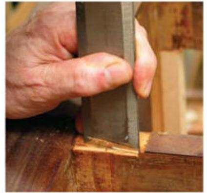
**Build out substrate.** Often the drawers have worn into the front rail of the chest so that the wear has to be built out before the veneer can be replaced. Here, I'm using a chisel to cut a flat surface for the patch to be glued on to.
