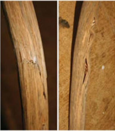
**Tension shear & compression.** In tension shear (left), the fibers simply tear during bending. A compression failure (right) – where fibers wrinkle instead of bend – typically occurs on an inside curve.
