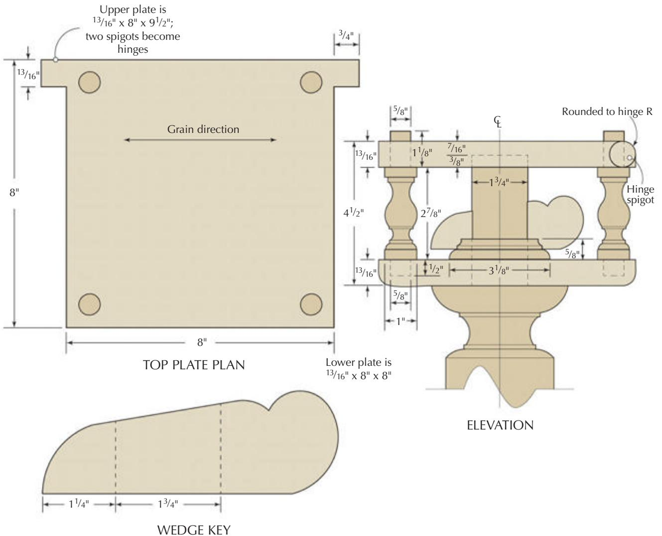
the latch tongue. The keeper needs to be mortised into the top face of the upper plate, on the arris opposite the hinge end. First measure and mortise in the edge lip. Then position and scribe around the face lip of the keeper. In my case, I have the stylish curves to deal with, so I use carving gouges to chop the edges of the mortise.
