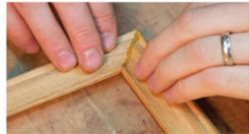
**Hold tight.** With nothing more than finger pressure pushing the joint together, hot hide glue will hold the miter joint tight as it dries.
