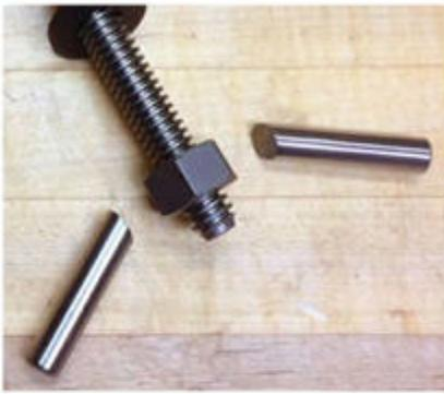
**Ready for welding.** I chuck the handles in my drill press and buff them to a sheen using progressively finer grits of sandpaper. After welding, I apply gun bluing.
