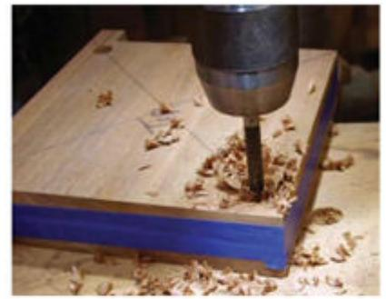
**Four corners.** Drill through the top plate in the package and into the bottom one, stopping  $\frac{1}{4}$ " from the press table (in other words, drill  $1\frac{3}{8}$ "-deep holes).
