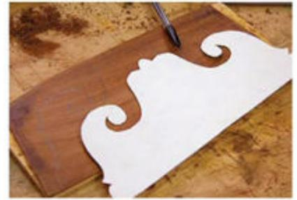
**Posterboard pattern.** I made this posterboard pattern by pulling dimensions off a photograph of the original. Dividers are handy for transferring key dimensions.
