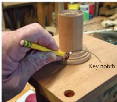
**Key mark.** With the lower plate and washer in place on the spindle, mark the bottom of the notch for the key.
