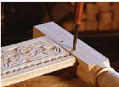
**Pinned.** Use a drawbore pin to test-fit the joint after drilling the holes in the tenon.
