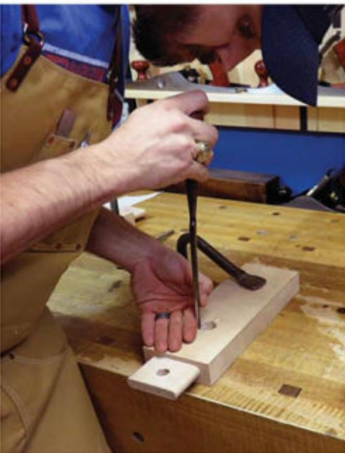
**Nut housing.** To house the nut on the threaded rod, chop out a mortise on the back of the rear leg. A 1" Forstner bit removes most of the waste; a chisel takes care of the rest.
