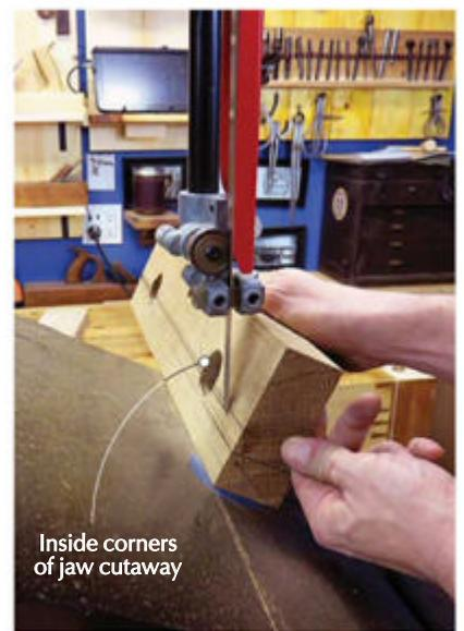
**Less is more.** Removing material on the outside of the jaws makes it easier to file, allowing you to add slope to your gullets if so desired.
