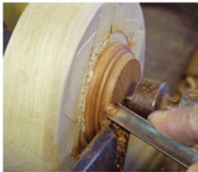
**Edge treatment.** After turning the washer blank round, use a skew and gouges to shape the edge to your liking.
