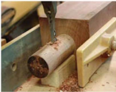
**Plunge cut.** After aligning the bit to the center of the blank and supporting the spindle in the scrap's trough, drill the mortise.
