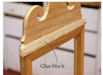
**Crest support.** The crest is not very thick, so adding a glue block on the back is wise. Make sure to taper it on the top and sides so it's inconspicuous.
