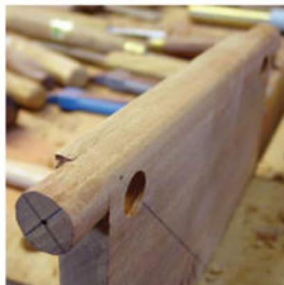
**Plane work.** I use a block plane to round over the edge between the spigots.
