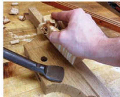
**Depressing work.** Using a block plane, start forming the lateral spring joint by taking a few light passes in the middle, working your way to the edges with each pass. The resulting depression should be approximately  $1/16$ " when complete.
