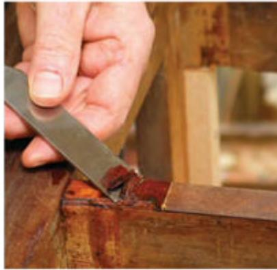
**Separate the veneer.** With the hide glue crystallized, it's usually easy to separate the veneer from the substrate using a chisel. To avoid cutting into the substrate and losing control, I prefer that the chisel be dull.
