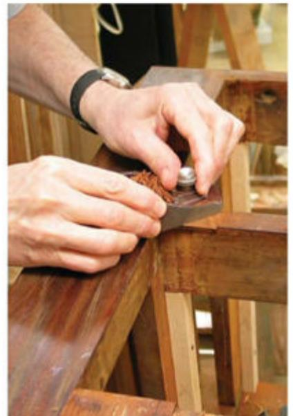
**Trim the veneer.** Because the veneer used on this chest-of-drawers was considerably thicker than modern veneer, I used solid wood for the patches. Then I trimmed each patch level with a hand plane.
