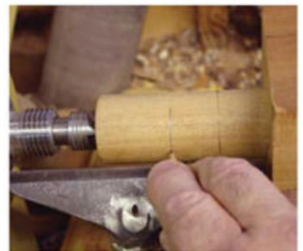
**Slot layout.** Using the measurements pulled from the key, mark the location on the spindle for the key slot.
