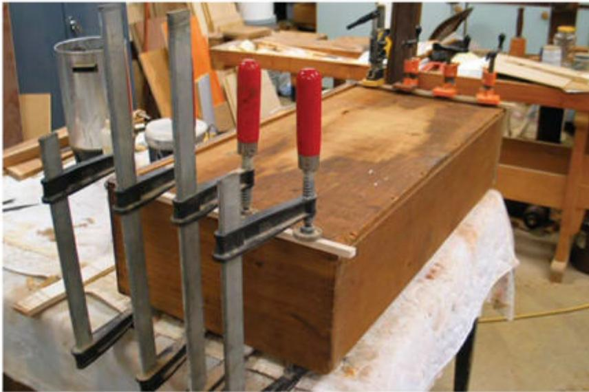
**Glue on new.** With the bottom of the drawer side perfectly flat, it's easy to glue on new wood, followed by trimming it with a handplane so the drawer slides easily on the new runners.
