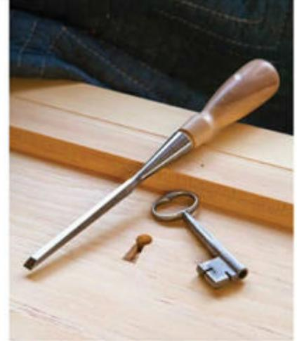
**Keyholed.** *The only tough part about installing a crab lock is cutting a well-placed and crisp keyhole. I bore the hole for the round part of the key. Then I cut the remainder with a chisel.*
