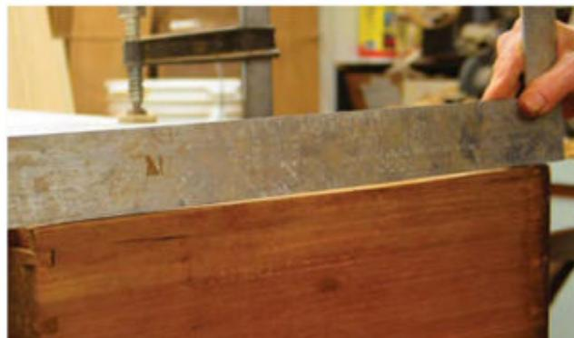
**Worn drawer sides.** Like the runners, the bottoms of the drawer sides also wear concave after many years of the drawers sliding in and out of a chest.
