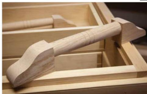
**Rasp the bone.** Then shape the ends of the lifts. This shape leaves plenty of meat for the screws to bite into.
