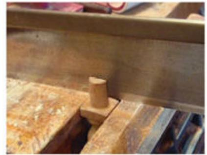
**Kerf.** Saw a kerf for a wedge to about  $\frac{1}{4}$ " above the tenon shoulder.
