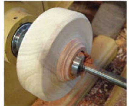
**Now drill.** Using the same  $\frac{1}{4}$ " Forstner bit you used to drill the hole in the top and bottom plates, drill a through-hole in the washer.
