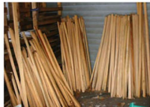
**Ripped & ready.** After riving the stock into eighths, I use a 3" resaw blade to follow the grain line and rip the pieces into bending stock, then leave it to air dry.
