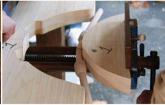
**Press.** Partial bends are done in a two-part press, with pressure supplied by a vise. Each half matches the shape I wish to accomplish.
