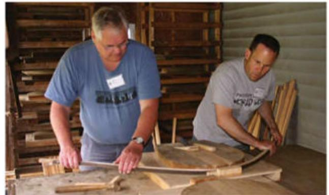
**A little help.** With two people working, and a strap providing the neutral line to keep all the wood in compression, a steamed piece can be bent around a form all at once.
