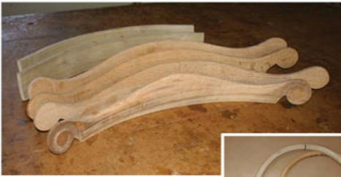
**Partial bends.** Crest rails, such as the various designs shown above, are partial bends, which are likely to be successful in a range of species. (Note: It's easier to do any carving or shaping while the wood is flat, then bend it.)
