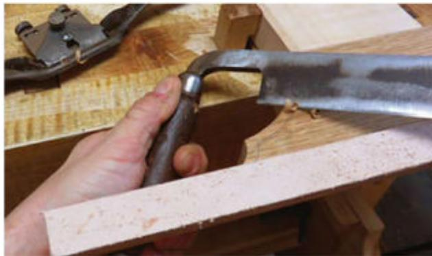
**Make it safe.** The 90° corners on the oak jaws can be sharp and dangerous. Adding a chamfer is made easier by securing the leg to your benchtop, allowing the jaw to overhang. This gives you access for easy shaping.
