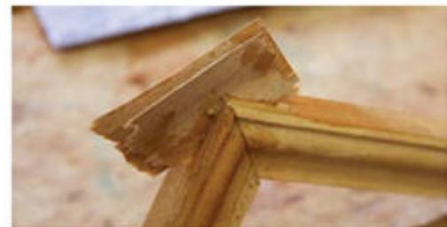
**Extra insurance.** Adding splines in the corners of mitered frames is an historic fail-safe in case the glued miter ever lets go.
