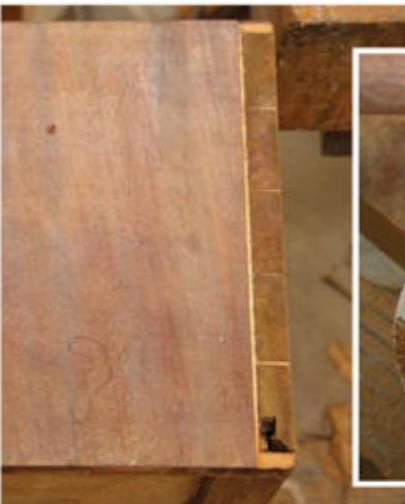
**Dovetailed end grain.** The glue bond of the veneer at the edges of the drawer fronts was weak because of the large percentage of end grain in the dovetail tails. Some of the veneer had popped off, leaving ragged edges. So I cut a straight line with the grain using a box knife just inside the damage and removed the waste with alcohol and a chisel.
