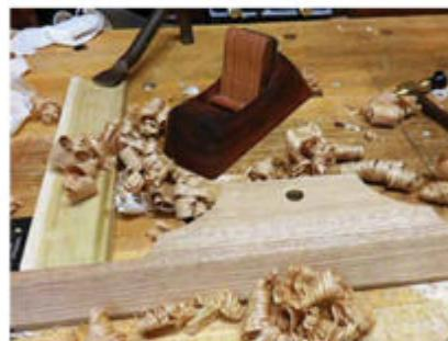
**Cleaning time.** I use a high-angle smoothing plane to clean up all of the jaw surfaces after rough shaping. The 60° tool works well on white oak, leaving behind a glassy surface.
