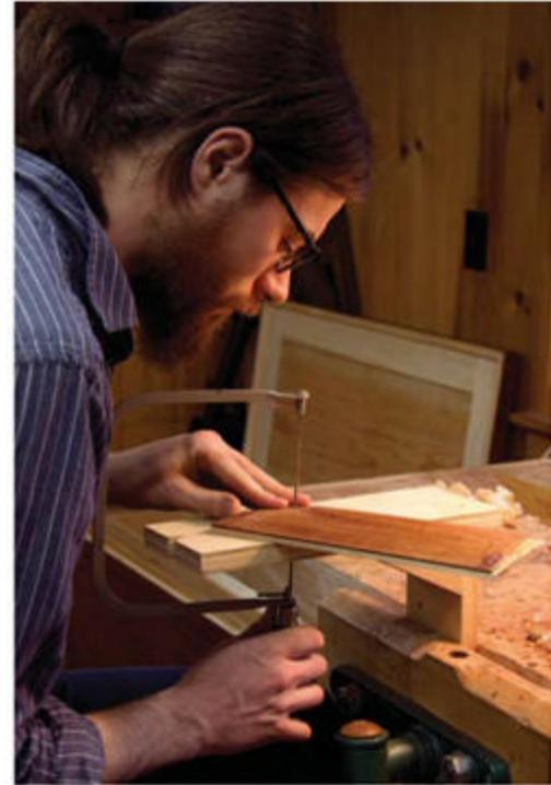
**Bird's mouth.** An L-shaped jig with a notch in the top surface for the saw blade makes it easy to saw out the scrolls of the crest, with plenty of support for the work. Because the bird's mouth is designed to clamp in a vise, it's easy to adjust the height as needed.
