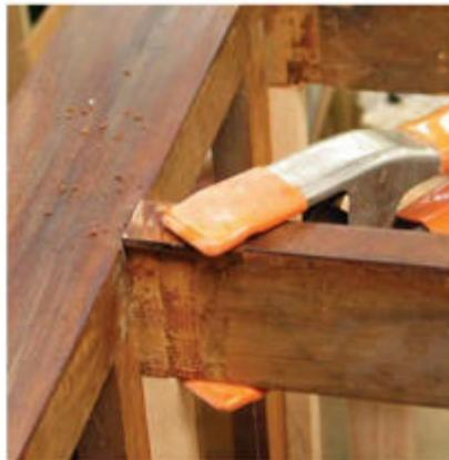
**Clamp the patch.** Thick veneer is actually very easy to work with. It can often be clamped without using a backing board.
