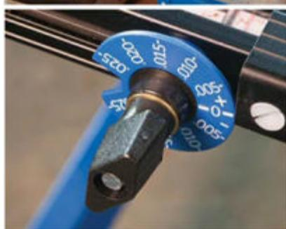
**Heavy-duty.** The steel base of the Kreg router table helps it stay put when you are running heavy stock, one of its many advantages over benchtop units. Plus, the simple micro-adjust feature allows you to make tiny changes with surprising and measurable ease.
