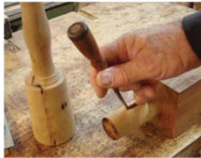
**Key angle.** Use a chisel to cut the slope for the wedge key's slot, angling down from the wider side of the mortise.
