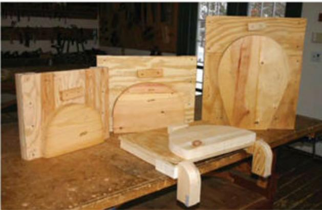
**Forms.** For complete bends, I use a form that matches the shape I wish to accomplish. The block at the top of each holds a wedge in place.
