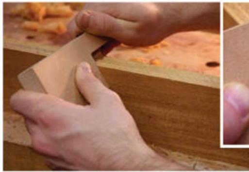
**Tilt into it.** By leaning the top of the scratch stock forward, the cut magically becomes smooth. If you're bouncing off your tracks, slow down and tilt forward more.
