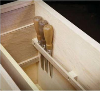
**Rack at the back.** This simple rack can hold a variety of tools. My other favorite form of rack is a board that is poked with 1/2"-diameter holes on 1/8" centers.
