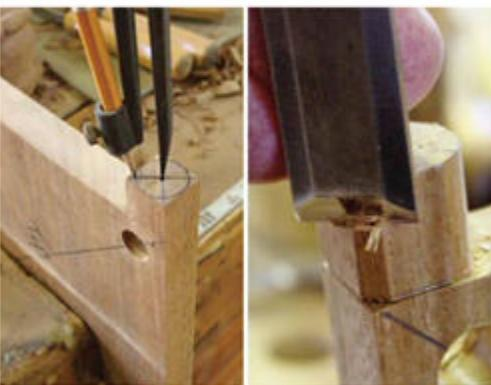
**Scribe, then shape.** After marking a centered  $\frac{13}{16}$ " circle on each spigot, use a chisel to nick the baselines, then pare each one round.
