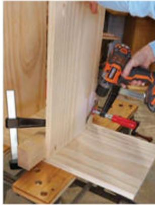
**Easy driving.** A block clamped in place to the layout lines makes it simple to hold the shelves perfectly in place as you drive the pocket screws. (Note: Because I'm using pine, a softwood, I used coarse-thread screws.)
