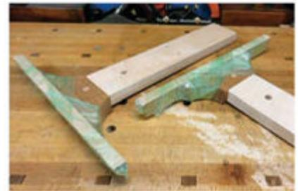
**Plastic fantastic.** Using plastic wrap is a great way to hold the leather strips in place where traditional clamps won't work. The angles on the jaw make any normal clamping setup difficult. Because a lot of pressure isn't needed for this application, plastic wrap is ideal.
