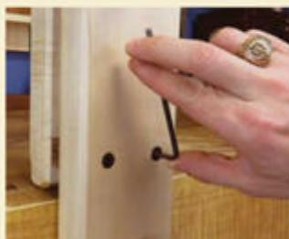
**No-headache tension.** By tightening each screw, you can increase the tension on each end of the jaws' spring joint. Snug the screws down until a standard handsaw can be supported without any assistance from the wing nut. Adjust the hinge as needed for seasonal changes and wear.
