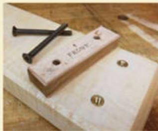
**Consistent alignment.** Two Allen-head screws pass through the hinge assembly and screw into threaded brass inserts. I like to mark the orientation of my hinge; it helps keep the jaw alignment consistent if you have to disassemble and reassemble the vise.
