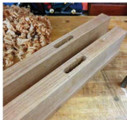
**Plumb the depths.** I hog out most of the mortise waste on the underside of the jaws using a 5/8" Forstner bit at the drill press, then use a wide chisel to clean up the edges and corners. The valleys created by the bit make a good guide to create plumb walls.
