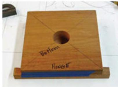
**Drilled & marked.** After finding the center point on the exposed faces of the taped-together top and bottom, drill a  $1\frac{3}{4}$ "-diameter hole through the bottom and into the top; the bit should stop  $\frac{3}{8}$ " above the table.
