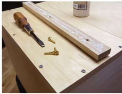
**Resist rot.** Either make your rot strips impervious to water (plastic would work, too), or make them so they will rot off immediately by using pine and iron nails. Either way works.
