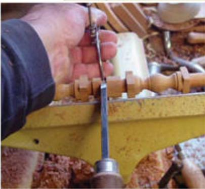
**Balanced balusters.** Strive to have the turnings match, but 18th-century examples prove they needn't be exact. The tenons, however, must be  $\frac{3}{8}$ " diameter for a good fit.
