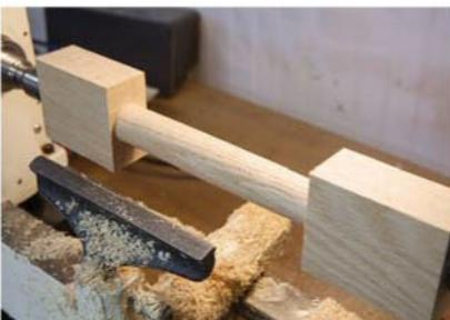
**Turn the bone.** The center section of the dog bone is turned down to 1" diameter. Then remove the piece from the lathe.
