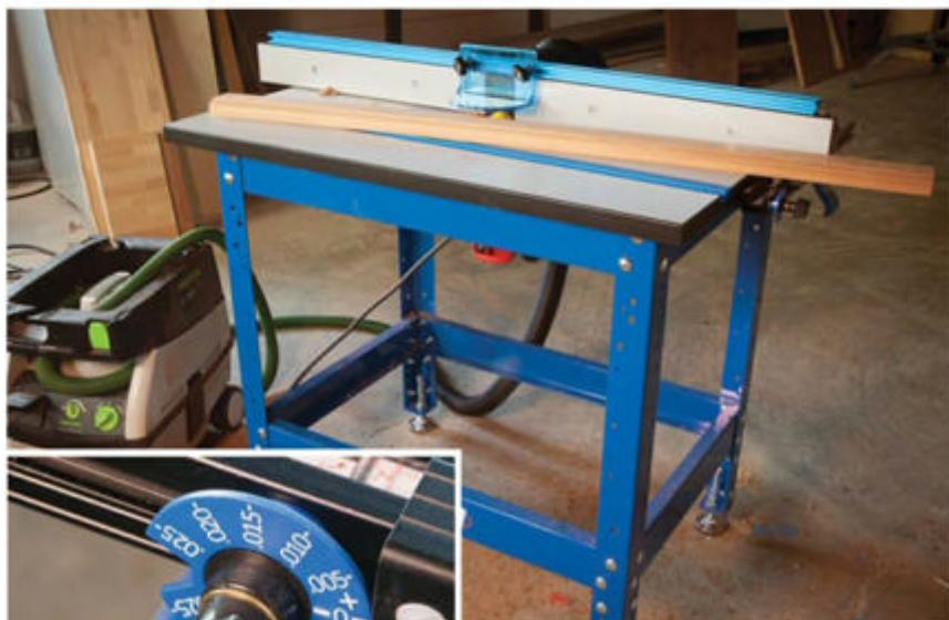
**Heavy-duty.** The steel base of the Kreg router table helps it stay put when you are running heavy stock, one of its many advantages over benchtop units. Plus, the simple micro-adjust feature allows you to make tiny changes with surprising and measurable ease.
