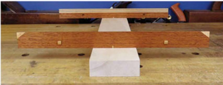
**Straight & square.** After roughing out the stock and letting it acclimate, I check for twist using a set of winding sticks. I square the stock using handplanes before laying out the joinery.
