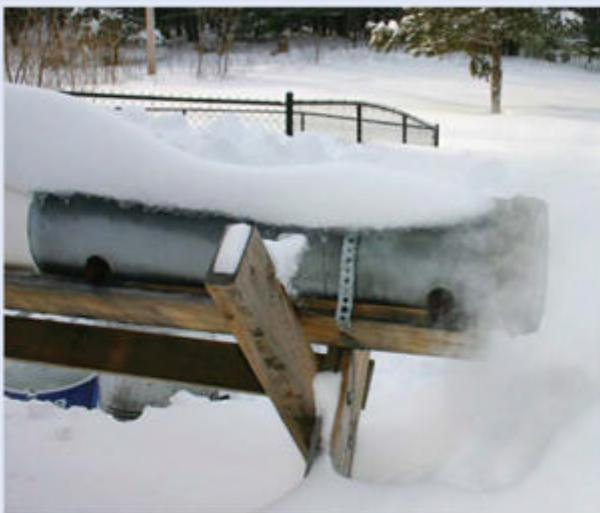
**Excellent insulator.** The PVC pipe provides such good insulation that snow remains on top in the winter even when the steam setup is going at full power.
