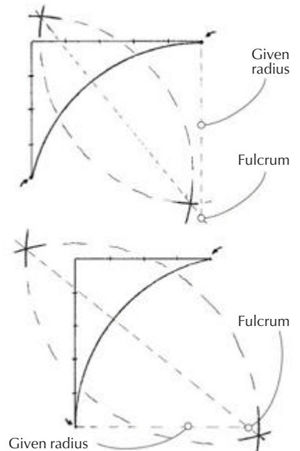
**Find the fulcrum.** The given radius springs from the end where the arc runs tangent to vertical or horizontal. Use the end points marked by arrows to draw a pair of intersecting arcs. Connect the intersections with a line and extend it. Where it crosses the given radius is the fulcrum.
