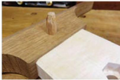
**Classic joinery.** A  $\frac{5}{8}$ " dowel is used to draw bore the joint. I used an offset of approximately  $\frac{1}{32}$ "; hardwoods don't require a lot. Using the  $\frac{5}{8}$ "-diameter dowel greatly reduces the odds of it splitting while being hammered home.
