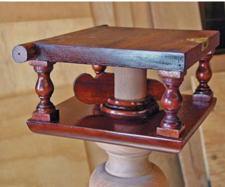
This clever & traditional wooden mechanism allows tabletops to tilt and rotate.
