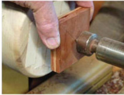
**Washer mount.** Put a scrap face plate on your lathe's head stock and apply double-sided tape to secure the washer blank. Use the tailstock to locate the center of the blank, then advance the tailstock to secure the blank to the tape. Now place a caul between the blank and tailstock to press the blank firmly in place.
