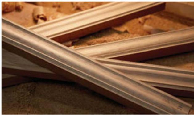
tom moulding profiles without fancy tools. I trace out the profile onto a cutter blank (a piece of an old handsaw blade) with a fine-point Sharpie. Then it takes only a couple minutes of file work to shape the profile (keeping a square edge will help in use). Some folks use slipstones to finish shaping the profile but, because we're using this scratch stock on long grain that is tame, I have not found that extra sharpening step to be necessary.
