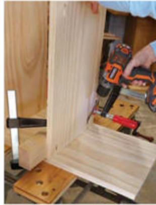
**Easy driving.** A block clamped in place to the layout lines makes it simple to hold the shelves perfectly in place as you drive the pocket screws. (Note: Because I'm using pine, a softwood, I used coarse-thread screws.)
