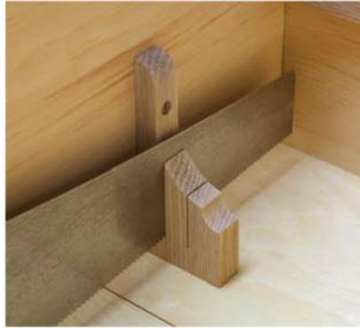
**Quick saw till.** Kerf the block of wood for the saws, then shape the block so it looks nice (top). Then screw it to the side of the carcass and to a bottom board (bottom).
