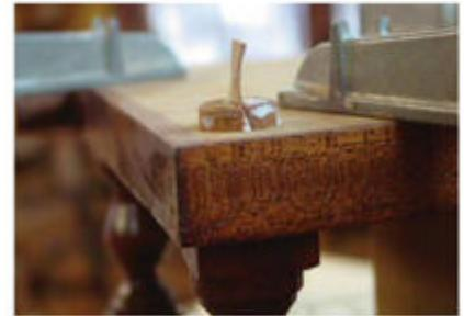
**Wedge.** After assembling the mechanism, glue and insert the wedges perpendicular to the grain of the upper plate.
