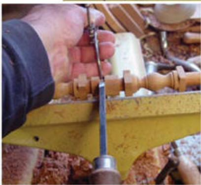
**One blank; two balusters.** This 1" x 1" x 10" blank will yield two balusters.
